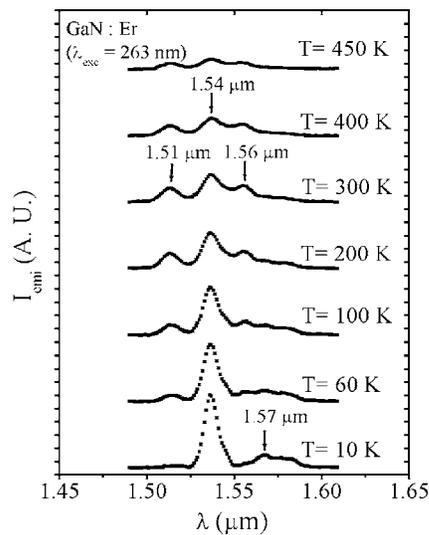
FIG. 2. Comparison of the PL spectra of the IR emission in Er doped GaN for  $\lambda_{\text{exc}}=263$  nm between 10 and 450 K.
