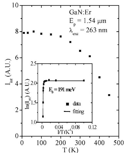
FIG. 3. Integrated PL emission intensity of the 1.54  $\mu\text{m}$  emission of Er doped GaN between 10 and 450 K for  $\lambda_{\text{exc}}=263$  nm. The inset is an Arrhenius plot of the integrated PL intensity of the 1.54  $\mu\text{m}$  emission.
