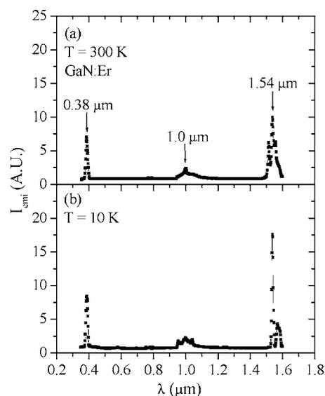
FIG. 1. PL spectra of Er doped GaN covering a broad spectral range from UV to IR for  $\lambda_{\text{exc}}=263 \text{ nm}$  at (a) 300 K and (b) 10 K.
