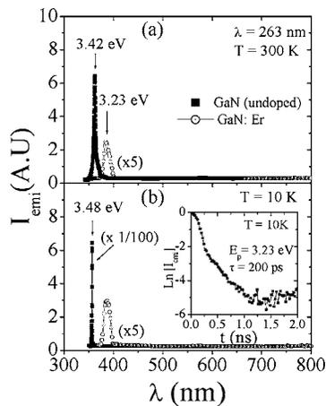
FIG. 4. Comparison of the band edge emission of undoped and Er doped GaN at (a) 300 K and (b) 10 K for  $\lambda_{\text{exc}}=263$  nm. The inset is the temporal response of the 3.23 eV emission intensity in Er doped GaN at 10 K.
